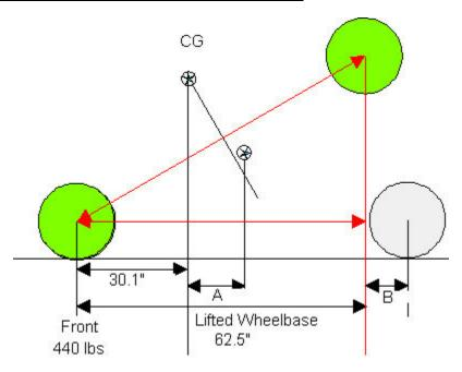
The diagram above shows the rear-end of a motorcycle lifted off the ground and what effect that has on the movement of the Center of Gravity towards the front of the bike. The diagram shows a lift considerably greater than 1 foot in order to clearly demonstrate the concepts described.
