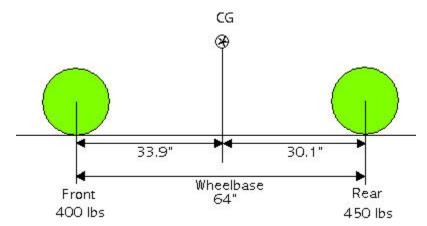
Repeat the measurements with a rider in the saddle. You will find that the Center Of Gravity has moved towards the rear of the bike.
