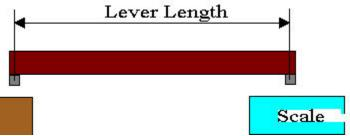
Before you place the wheel on the board note the weight on the scale. Let's say it shows 2 pounds. You then place the front tire on the board and measure the distance from the point the board contacts the scale to the center of the contact patch of the tire. Let's say that turns out to be 10 inches. 10 divided by 24 is .417, thus, 41.7% of the weight of the wheel will be on the end of the board away from the scale and 58.3% will be on the scale itself.
